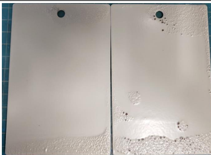
Powder coat over Corrosion Cure with mild rinse
