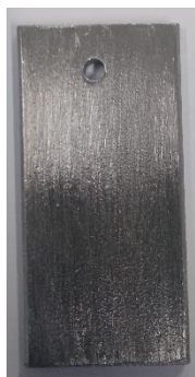
Figure 3. Image of untreated steel coupon S3(2) before Corrosion to Metals Test.
